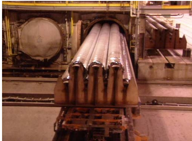
Master rolls being loaded into an « Autoclave » for curing
