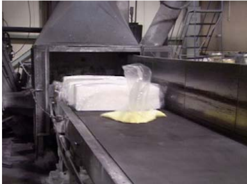
Raw material being fed into Banbury
