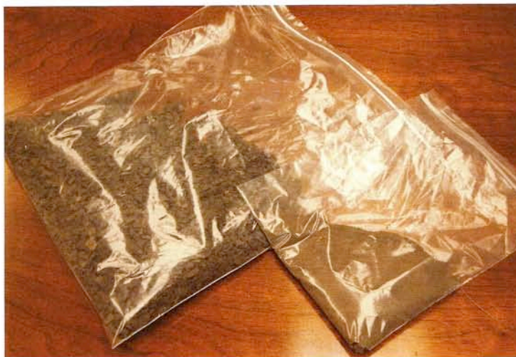
An EPDM membrane following the grinding process
